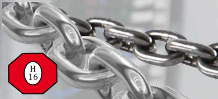
High-quality galvanized PEWAG HEO-EN 818-7-T GZN chain with 6-fold safety factor. Provided with a minimum surface hardness of 380 HV. This chain even has a higher surface hardness than the EN 818-7 and ISO 3077 standard, which improves the wear resistance. PEWAG chain license plate (H stamp) H16
